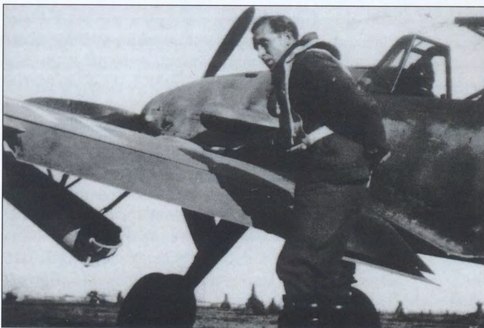
The firing cable was attached to the rear inner support strut of the launcher, and from there fed round through the backplate of the tube. This weapon was nicknamed the 'stovepipe' by the Jagdwaiffe crews that used them in combat
