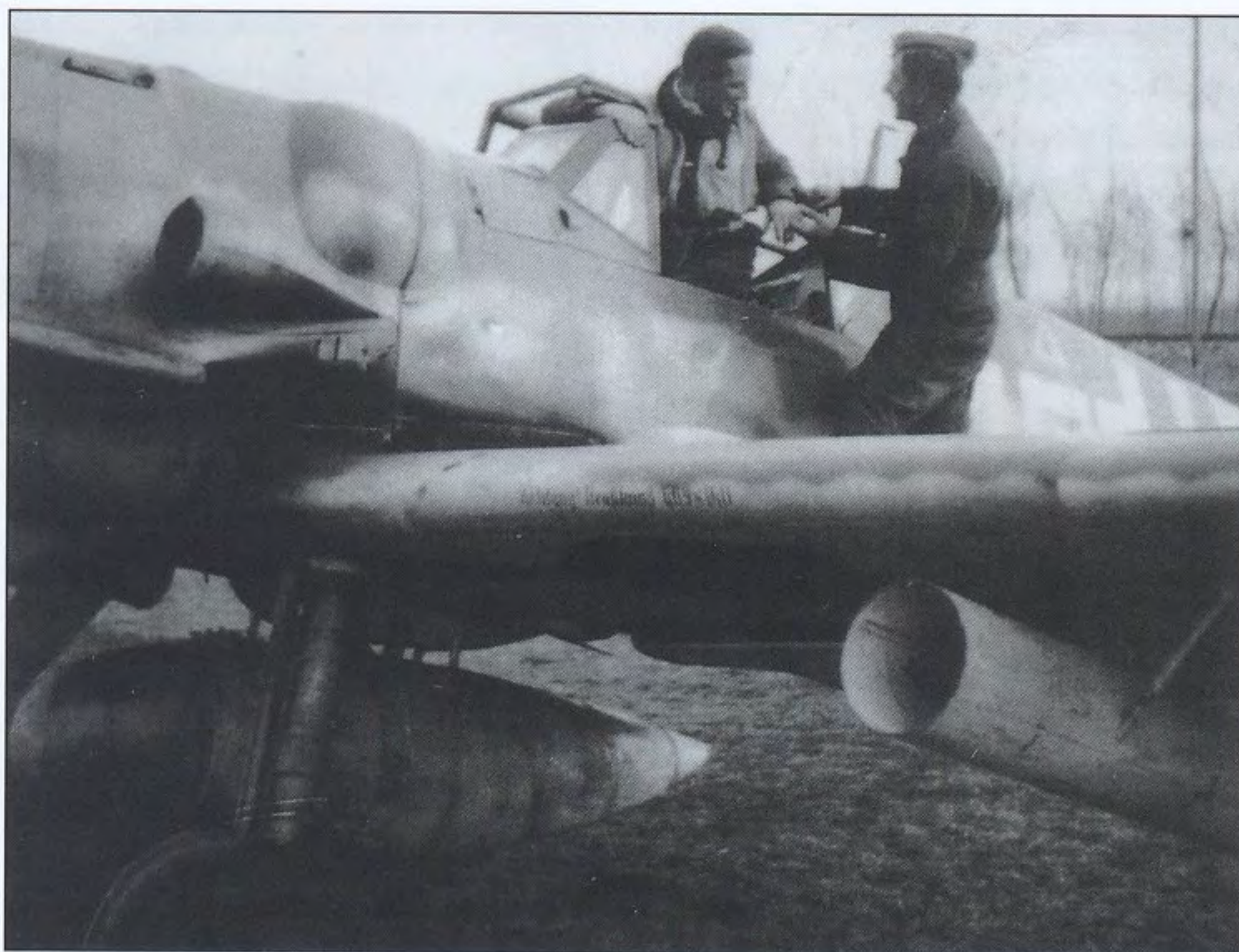
The business end of the underwing launcher for the 210 mm air-to-air rocket. The nose of the missile can just be seen inside the tube
